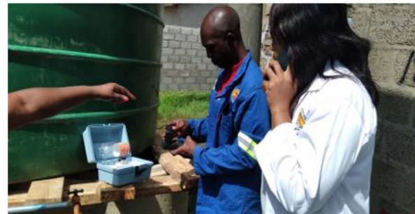
Checking for chlorine residual in the installed tanks
